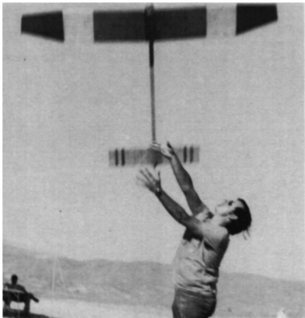
Making a perfect hand-launch of his Mach Zu, Glen Schneider releases the ship at a steep angle in a slight right bank—note angle of trailing edge of stab with the horizon. The 735 sq. in. ship is powered by a K&B Schnuerle Class C engine. See text for launching techniques.
