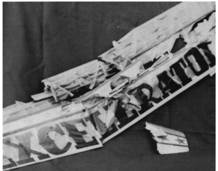
Problems increase with speed, as badly damaged wing attests. Wing flutter at high speed caused this havoc to 1175 sq. in. wing of author's OS Max 65 RR Schnuerle powered Excelsior D Gas design. Too little incidence did it in—see Problem 3 in the text. And the wing was a toughie—full geodetic ribs, spruce turbulating spars, silk covering.
